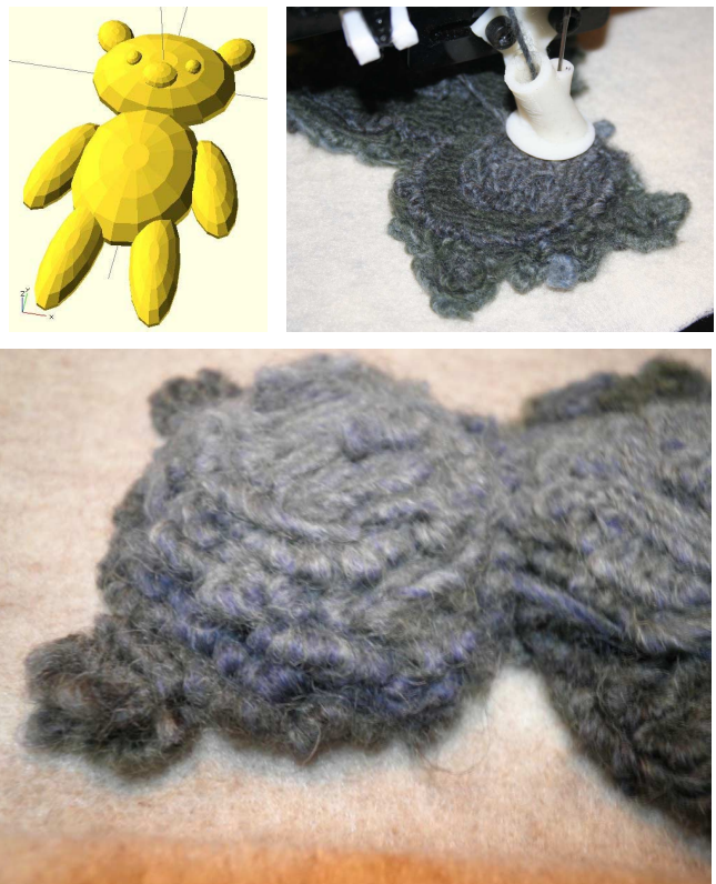
Figure 1. A 3D Printed Teddy Bear. Solid model (top left), printing in progress (top right) and result (bottom).
