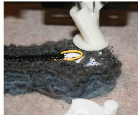
Figure 8. Partially printed arm example showing embedded components. Here we can see an embedded black nylon mesh tube (left) which holds a yellow tendon wire. This wire loops around a bolt which attaches the (white) assembly under it that is being printed over at this point. This assembly contains an embedded metal nut, nylon mesh to spread forces from the hard attach point and 3D printed stiffening material.
