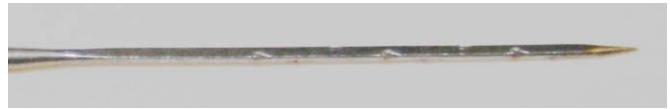
Figure 2. The felting needle used in this work is triangular with barbs in the form of notches placed approximately 2mm apart around the needle.
