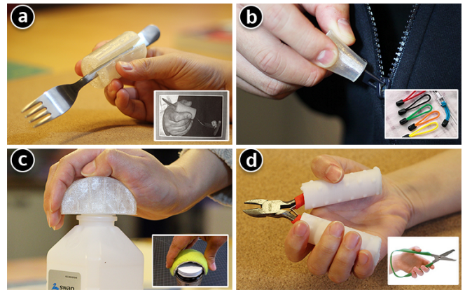
Figure 17. Replicated wrapper/extension examples. NinjaFlex was used for the fork wrapper (a), zipper handle extension (b), and the bottle wrapper (c). Nylon-based soft material was used for the cutter.
