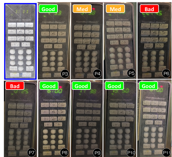
Figure 6. Examples of the attached overlay performed by the participants. For P4 and P5, slight offset did not affect using the appliance. An exact alignment is shown in the top left corner.
