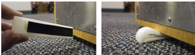
Figure 7. Embedding a piece rubber to make a functional door stop. Medley allows the creation of this embeddable (DOW=2) by simple drawing and extruding a line.
