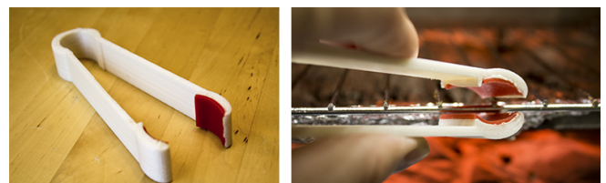
Figure 11. Embedding scraps cut from a silicone oven mitt into a pair of tongs makes it possible to be used with hot objects.
