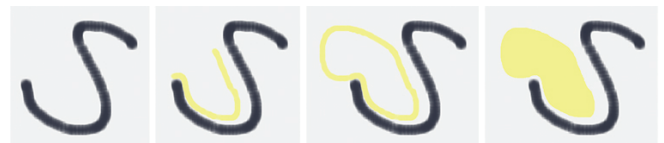
Figure 6. Lasso-selecting an area of clearance around the tip of the hook (no structure generated here).
